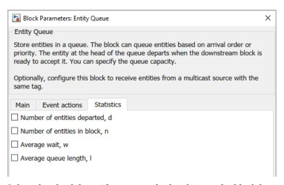
2 Select the check box. After you apply the change, the block has a new signal output port corresponding to that statistic.
