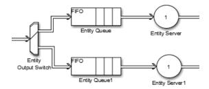
By looking at the entity connection lines alone, you cannot tell which queue block's **IN** port an entity arrives at. Instead, you need to know more about how the one-to-two block (Output Switch) behaves and understand the outcome of certain run-time decisions.
