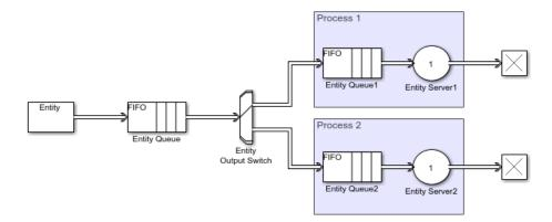
Connecting two queue-server pairs in parallel, in which a copy of each entity arrives at each, can represent a multicasting scenario, such as sending a message to multiple recipients. Note that copying entities might not make sense in some applications. For an example, see "Broadcast Entities using Entity Multicasting".
